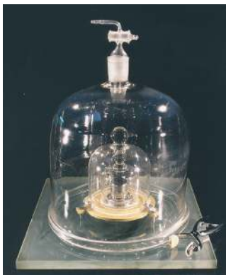
The international prototype of the kilogram, \mathcal{K} , the only remaining artefact used to define a base unit of the SI.
